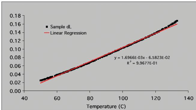
Figure 2: Sample displacement against temperature for a polycarbonate.
