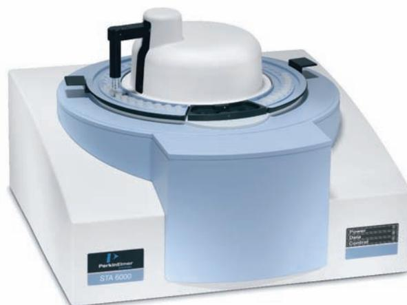
Figure 7. STA 6000 with 45-position autosampler.
