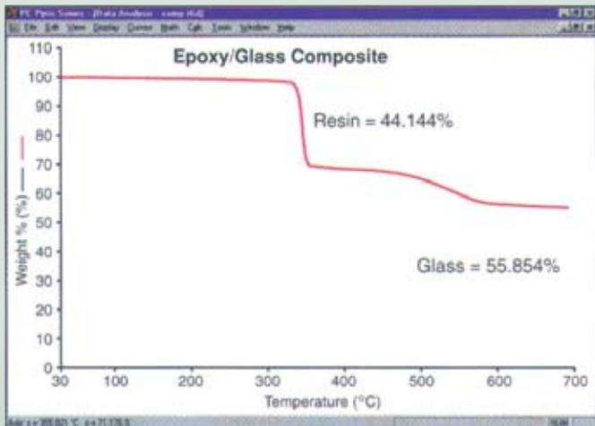
Figure 1. Physical properties of epoxy/glass composites are affected by the resin-to-glass ratios. Since glass is generally less expensive than resin, manufacturers strive to maximize glass content while maintaining the desired performance properties of the composite. The TGA 4000 is used to determine the percentage of resin and glass in the composite.
