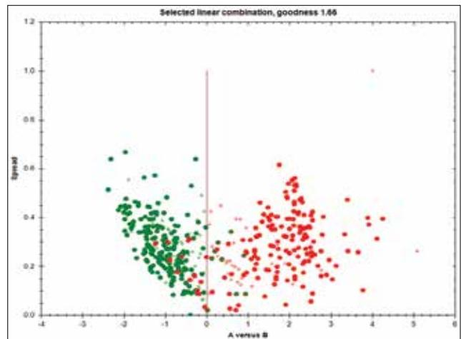
The PhenoLOGIC software plug-in makes it easy to create optimized algorithms. Click on a few objects to teach the algorithm to recognize the different types, then PhenoLOGIC calculates a linear classifier and identifies them in all images.
