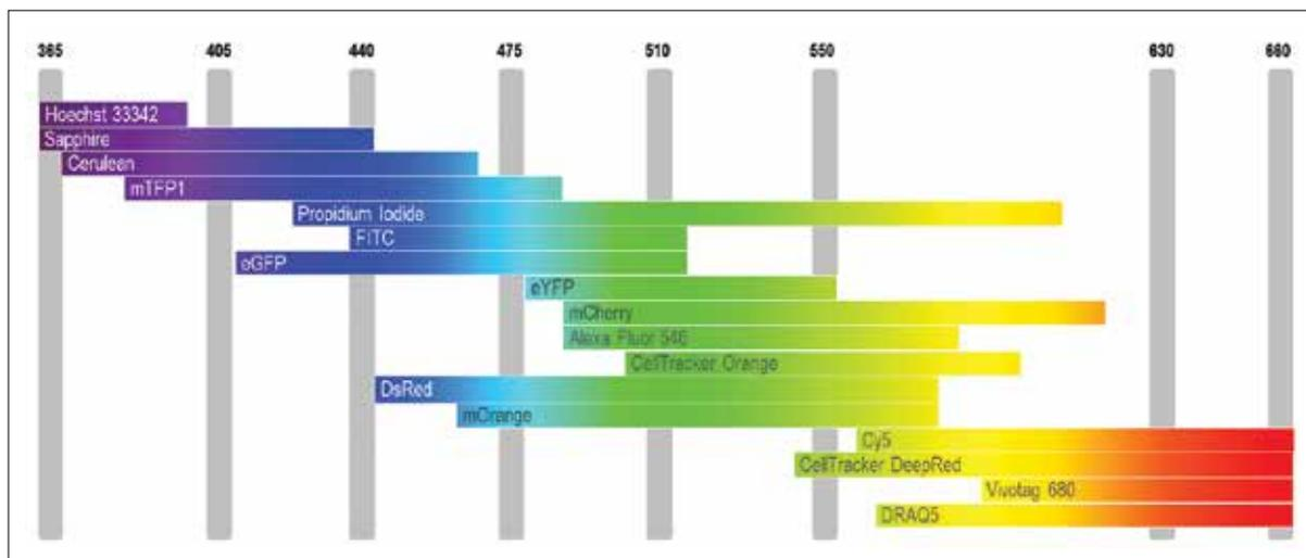
Up to eight LEDs excite a wide range of fluorophores, from UV to NIR, including DNA stains, live-cell stains, fluorescent proteins, and typical covalent labels. Some popular dyes are shown here.
