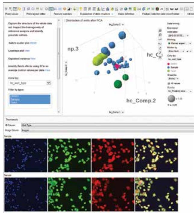
High Content Profiler software's powerful visualizations help turn data into actionable insights. This illustration shows a principal component (PCA) plot for exploring the phenotypes caused by positive controls (light green) and samples (blue).
